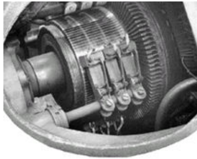
Figure 1. Typical DC Motor Brushes And Commutator
