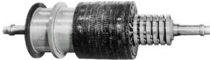
Figure 2. Rotary Converter Armature Showing Commutator And Slip Rings.
