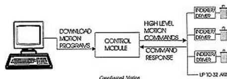
In multi-axis applications that do not require simultaneous motion, where only one motor moves at a time, it is possible to "multiplex" the step and direction pulse from one indexer to multiple drivers.
