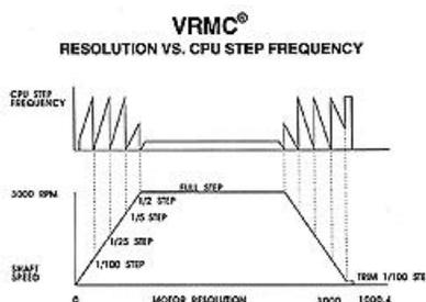
Microstepping is typically used in applications that require accurate positioning and a fine resolution over a wide range of speeds.
