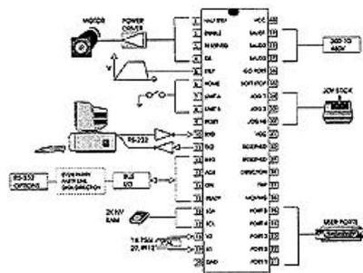
SMC-C24 Step Motor Control I.C.
