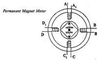
Unlike the other stepping motors, the PM motor rotor has no teeth and is designed to be magnetized at a right angle to its axis. The above illustration shows a simple, 90 degree PM motor with four phases (A-D). Applying current to each phase in sequence will cause the rotor to rotate by adjusting to the changing magnetic fields. Although it operates at fairly low speed the PM motor has a relatively high torque characteristic.
