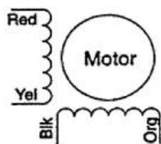
*4 Lead Unifilar Motor*
