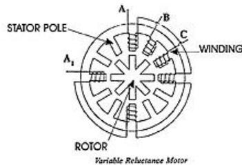
The variable reluctance motor in the above illustration has four "stator pole sets" (A, B, C), set 15 degrees apart. Current applied to pole A through the motor winding causes a magnetic attraction that aligns the rotor (tooth) to pole A. Energizing stator pole B causes the rotor to rotate 15 degrees in alignment with pole B. This process will continue with pole C and back to A in a clockwise direction. Reversing the procedure (C to A) would result in a counterclockwise rotation.
