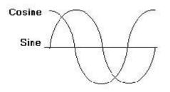
where the Sine and Cosine signal have a 90° phase shift from each other. Converting the resolver signal provides an absolute position signal within one revolution of the motor. The resolution of the converter depends mainly on the motor speed. The chart below shows the R/D converter specifications for a given speed range.
