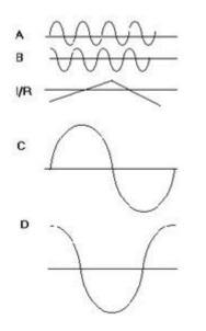
As shown, the A & B channels are interpolated while the C & D channels are used for absolute positioning in one revolution of the motor.
