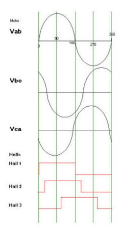
Some six-step drives incorporate this feedback for crude velocity sensing or course positioning. With sinusoidal current drives, they are sometime used along with incremental encoder feedback to give a course power-up position indicator. In servo drives, they are commonly used as current sensors to close the current loop. In other industry applications they are used for sensing the position of a crankshaft, cam, or other mechanical device.
