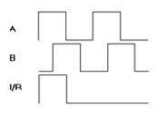
The encoder output can also have a compliment signal. The compliment signal aids in noise immunity. By detect the rising signal, or more positive going signal, the encoder resolution can be increased by a factor of 4. For example a 1024 line encoder with complimentary, or quadrature output, has 4096 counts per revolution.
